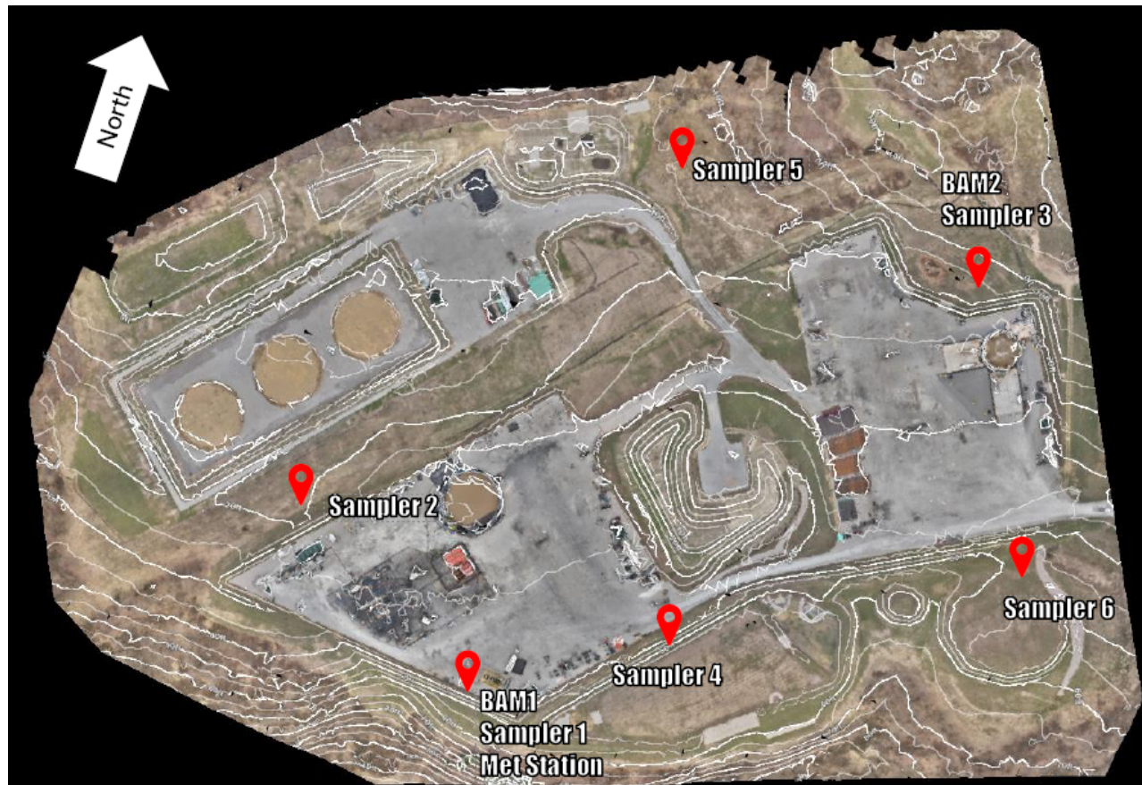
Figure AY-1. Aerial View of the MAM15 Complex and Monitoring Locations. Contour Lines Represent a 5 ft Elevation Difference.
