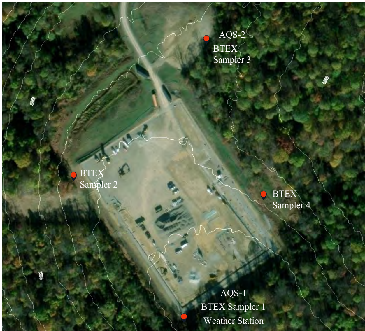
Figure AW-1. Aerial View of the Fatur Well Pad and Monitoring Locations (AQS-1 and AQS-2: PM2.5 Monitors, Met Station: Meteorological Measurement System, Sampler 1 – 4: Passive BTEX Sampling Location).
