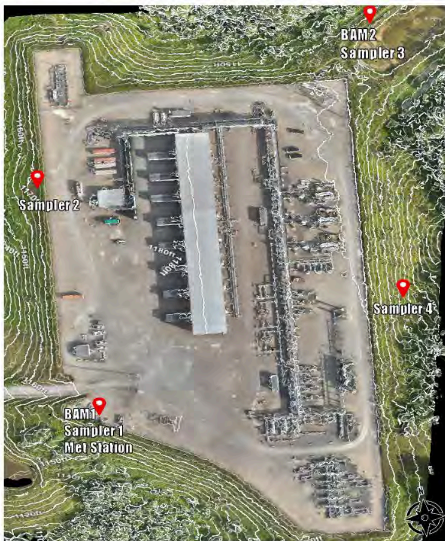
Figure AM-1. Aerial View of the Buckland Compressor Station and Monitoring Locations (BAM-1 and BAM-2: PM 2.5 Monitors, Met Station: Meteorological Measurement System, Sampler 1 – 4: Passive BTEX Sampling Location). Contour Lines Represent a 2 ft Elevation Difference.
