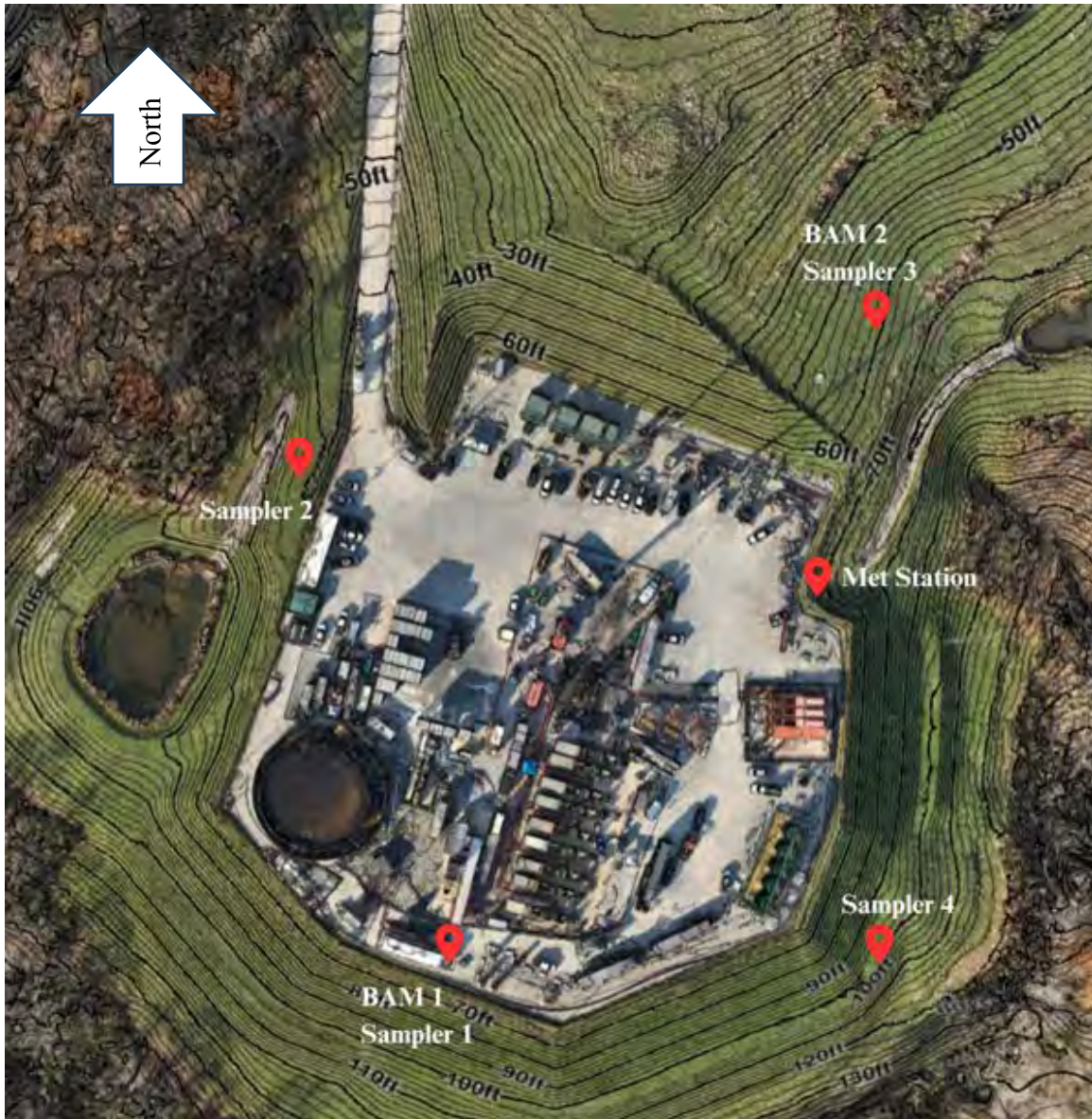
Figure AC-1. Aerial View of the RHL37 Well Pad and Monitoring Locations (BAM-1 and BAM-2: PM2.5 Monitors, Met Station: Meteorological Measurement System, Sampler 1 – 4: Passive BTEX Sampling Location). Contour Lines Represent a 2 ft Elevation Difference.
