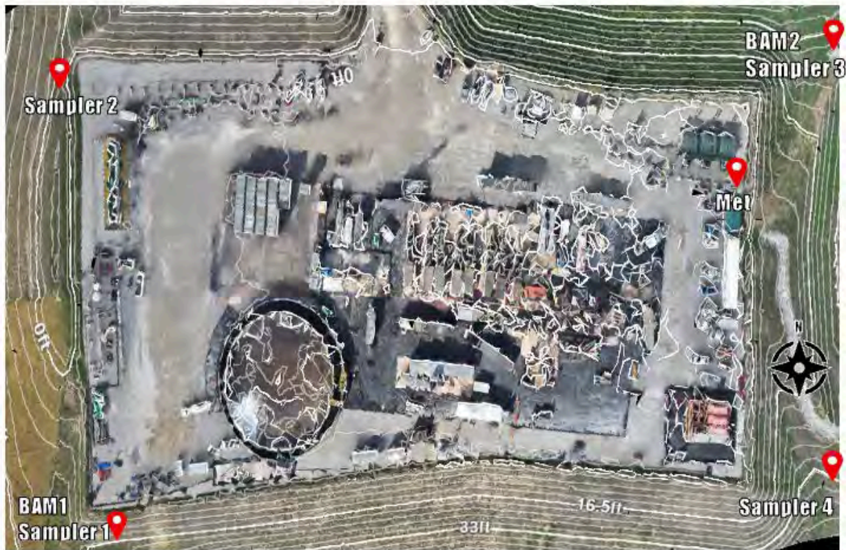
Figure AL-1. Aerial View of the NV113 Well Pad and Monitoring Locations (BAM-1 and BAM-2: PM 2.5 Monitors, Met Station: Meteorological Measurement System, Sampler 1 – 4: Passive BTEX Sampling Location). Contour Lines Represent a 5 ft Elevation Difference. Note: While all monitoring locations are depicted, markers may not be precise due to space limitations of the aerial image.
