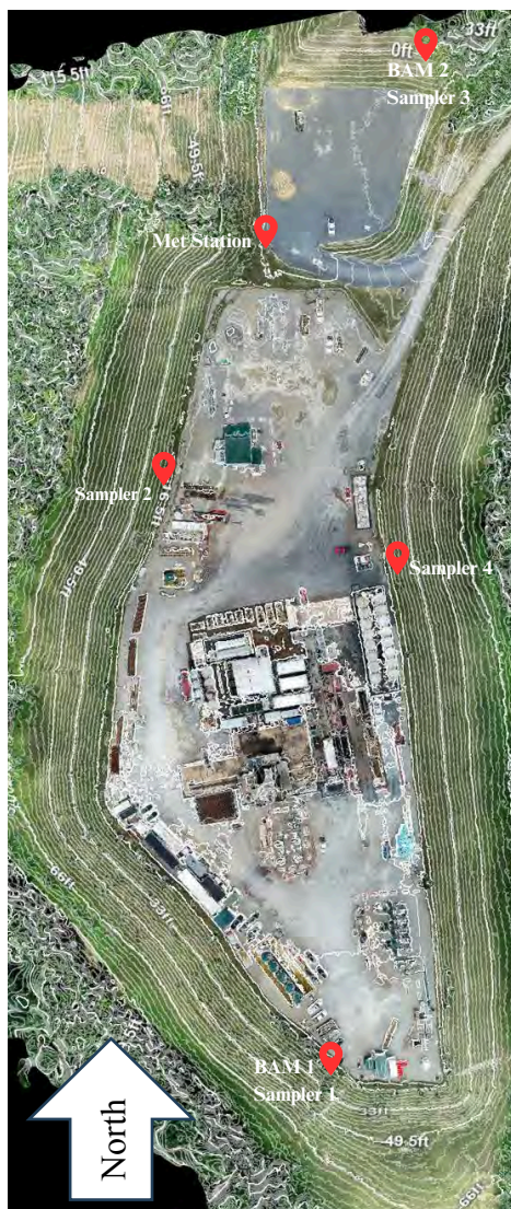
Figure AP-1. Aerial View of the WDTN5 Well Pad and Monitoring Locations (BAM-1 and BAM-2: PM2.5 Monitors, Met Station: Meteorological Measurement System, Sampler 1 – 4: Passive BTEX Sampling Location). Contour Lines Represent a 2 ft Elevation Difference. Note: While all monitoring locations are depicted, markers may not be precise due to space limitations.
