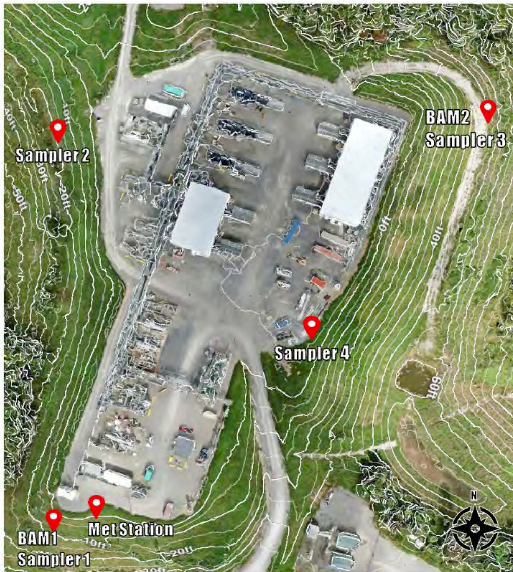
Figure AD-1. Aerial View of the Morris Station Well Pad and Monitoring Locations (BAM-1 and BAM-2: PM 2.5 Monitors, Met Station: Meteorological Measurement System, Sampler 1 – 4: Passive BTEX Sampling Location). Contour Lines Represent a 5 ft Elevation Difference.
