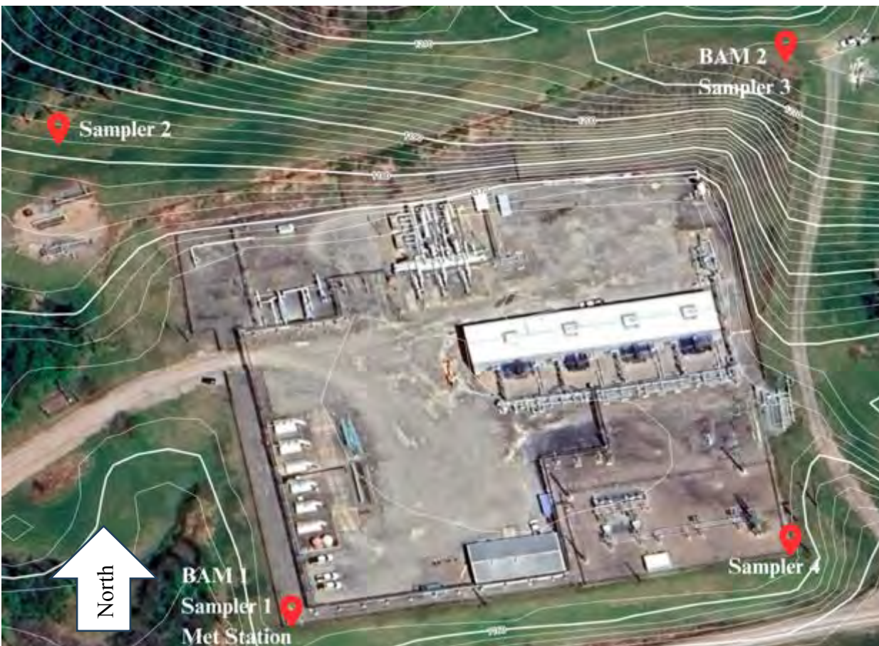
Figure AJ-1. Aerial View of the Mamont Station and Monitoring Locations (BAM-1 and BAM-2: PM2.5 Monitors, Met Station: Meteorological Measurement System, Sampler 1 – 4: Passive BTEX Sampling Location). Contour Lines Represent a 2 ft Elevation Difference.
