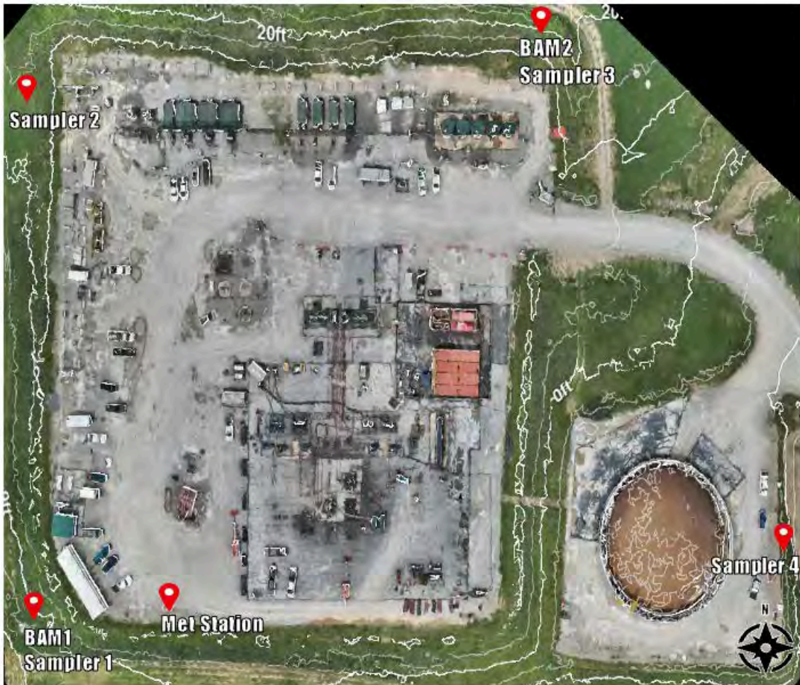
Figure AK-1. Aerial View of the BP6 Well Pad and Monitoring Locations (BAM-1 and BAM-2: PM 2.5 Monitors, Met Station: Meteorological Measurement System, Sampler 1 – 4: Passive BTEX Sampling Location). Contour Lines Represent a 210 ft Elevation Difference. Note: While all monitoring locations are depicted, markers may not be precise due to space limitations.
