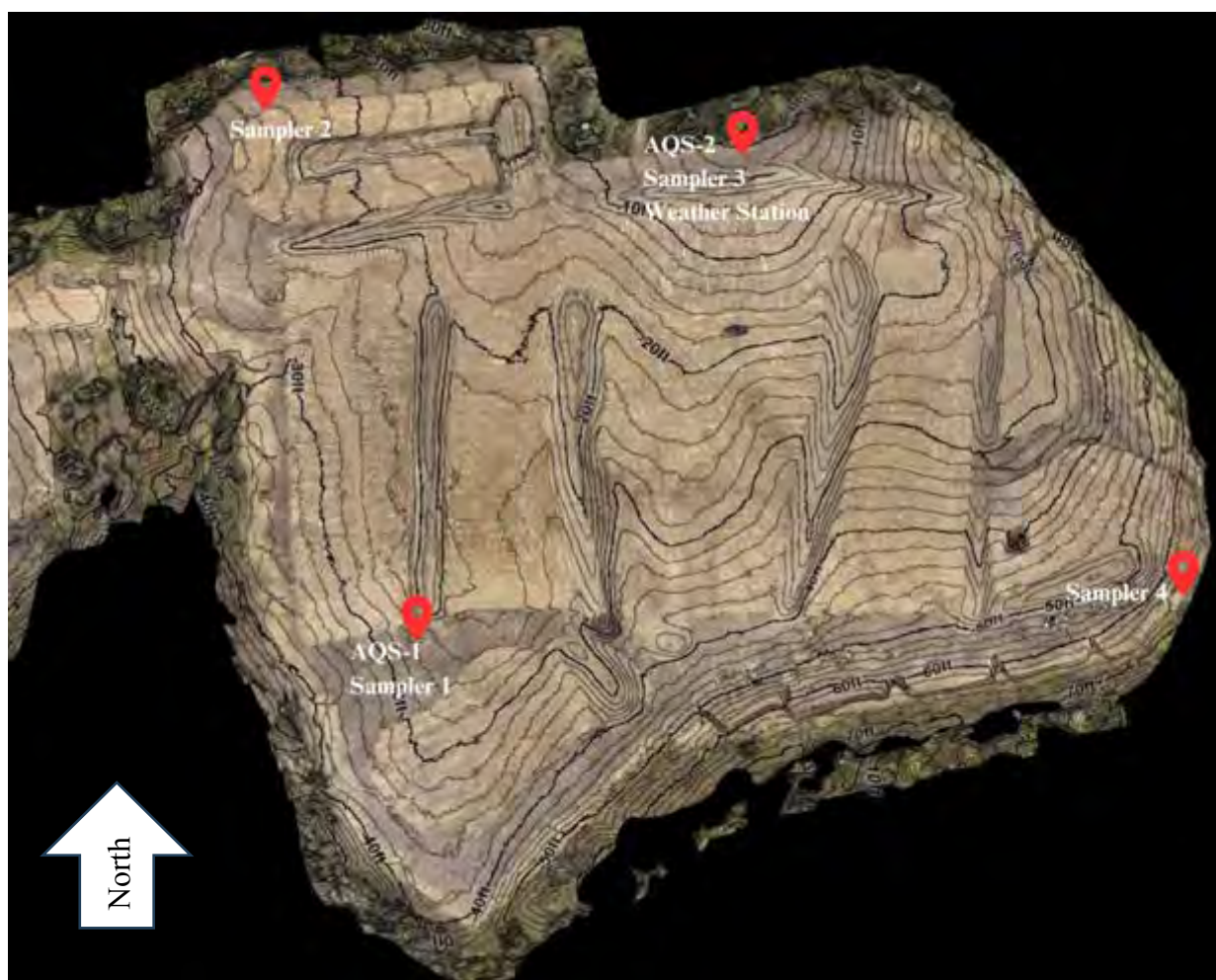
Figure AO-1. Aerial View of the MAM14 Well Pad and Monitoring Locations (AQS-1 and AQS-2: PM2.5 Monitors, Met Station: Meteorological Measurement System, Sampler 1 – 4: Passive BTEX Sampling Location). Contour Lines Represent a 2 ft Elevation Difference.
