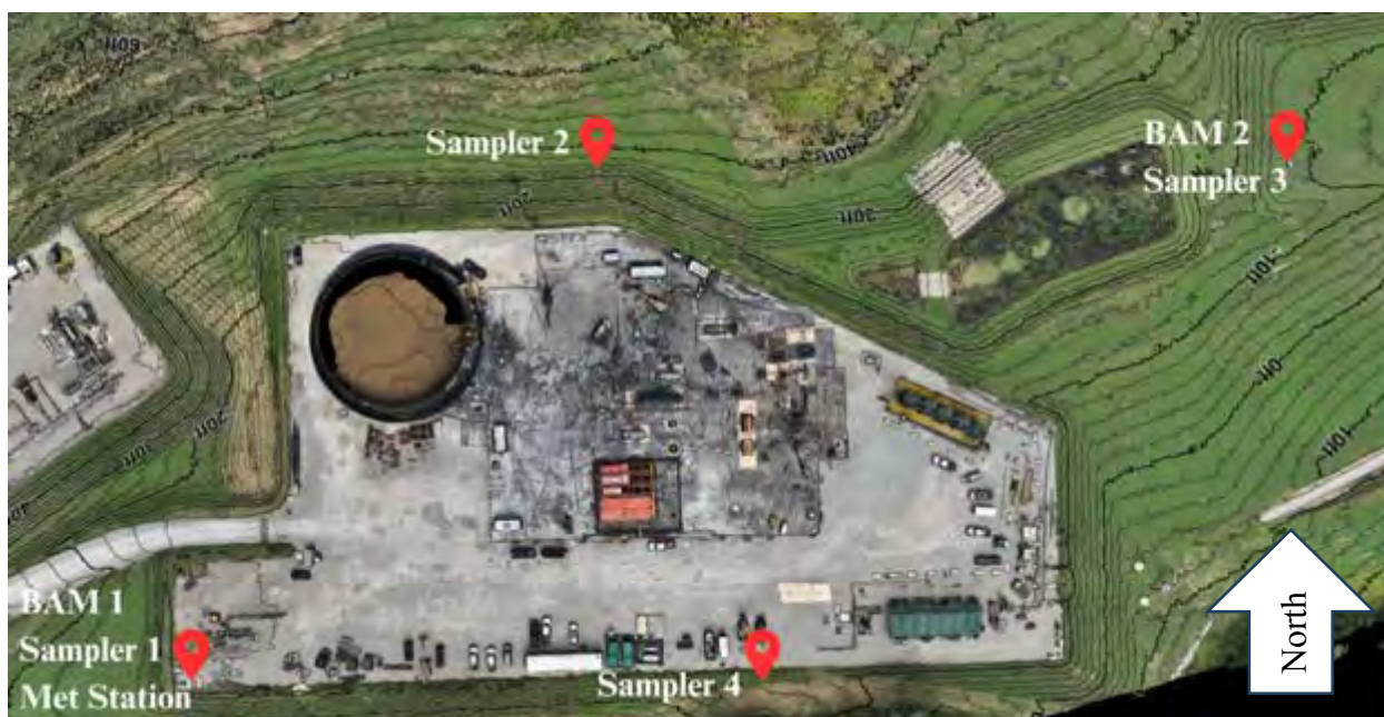
Figure AI-1. Aerial View of the MAM16 Well Pad and Monitoring Locations (BAM-1 and BAM-2: PM2.5 Monitors, Met Station: Meteorological Measurement System, Sampler 1 – 4: Passive BTEX Sampling Location). Contour Lines Represent a 2 ft Elevation Difference.
