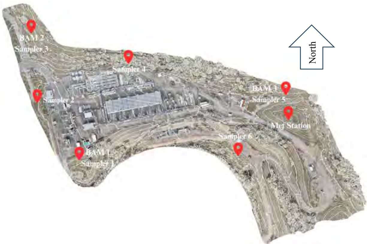
Figure AQ-1. Aerial View of the Majorsville Compressor Station and Monitoring Locations (BAM-1, BAM-2, and BAM-3: PM2.5 Monitors, Met Station: Meteorological Measurement System, Sampler 1 – 6: Passive BTEX Sampling Location). Contour Lines Represent a 2 ft Elevation Difference.
