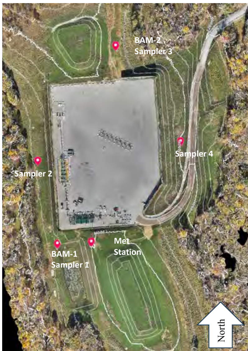
Figure AA-1. Aerial View of the NV110 Well Pad and Monitoring Locations (BAM-1 and BAM-2: PM2.5 Monitors, Met Station: Meteorological Measurement System, Sampler 1 – 4: Passive BTEX Sampling Location). Contour Lines Represent a 10 ft Elevation Difference.
